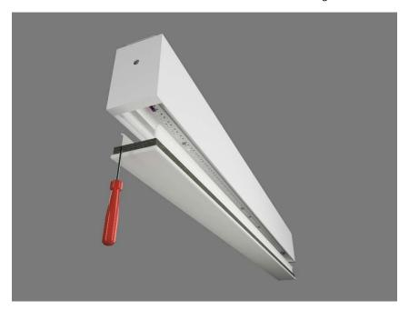
Step 1: Insert flat head screw driver into gap between lens and housing and carefully pry lens from housing (this will need to be done in multiple locations along one side of the lens to remove).
