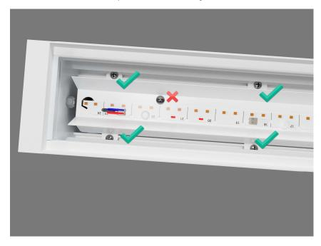
Step 2: Remove screws from gear tray that hold it to the extrusion (checked screws).
