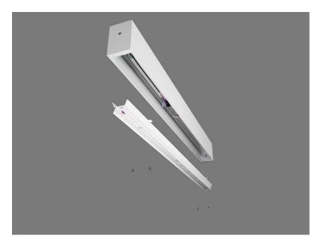
Step 3: Remove gear tray from housing and disconnect quick connects from driver. A new gear tray can be connected, and steps reversed to put luminaire back in working condition. Driver can also be removed and replaced during this stage.
